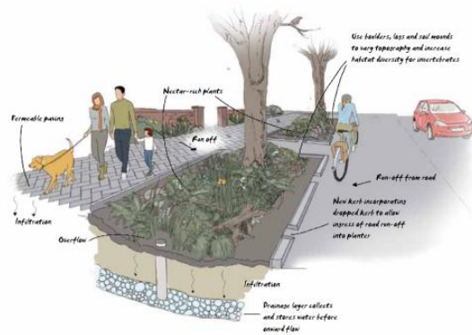
SuDS Bioretention Area (illustration courtesy of RSPB/WWT SuDS guide)
